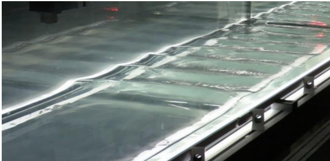
Figure 2: An experimental tidal bore with its undulation generated in the Pprime laboratory by a volume inversion method [Rousseaux et al. 2016] in an open water channel of rectangular geometry with a global flow reversal. The LED lit the secondary waves downstream of the tidal bore front from the channel sides through the glass windows.
