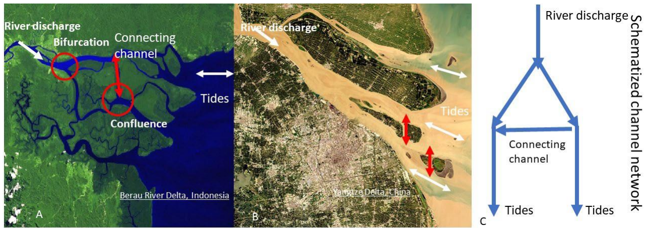
Figure 1: a) Map of the Berau Delta, Indonesia, showing the channel network and the presence of bifurcations, confluences and connecting channels. B) Same as a), but now for the Yangtze delta. C) Network of six channels as used in the morphodynamic model simulations. In some sets of simulation the connecting channel was absent, making this a three channel network.
